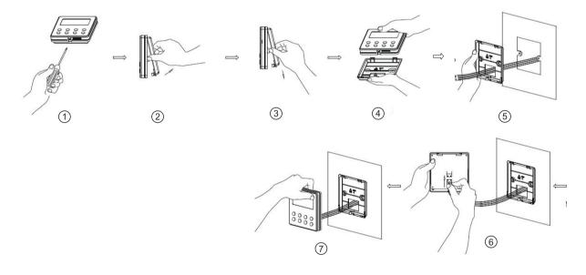
Fig.15 shows the installation steps of the wired remote controller, but there are some issues that need your attention.
